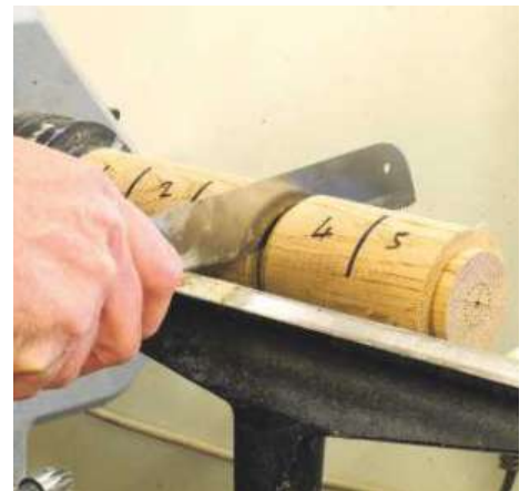
▲ Pic.6 Cut the lid away from the base using a fine-tooth saw. You could also do it under power if you are confident doing this with a parting tool, but the lid section is still quite a lump of wood
